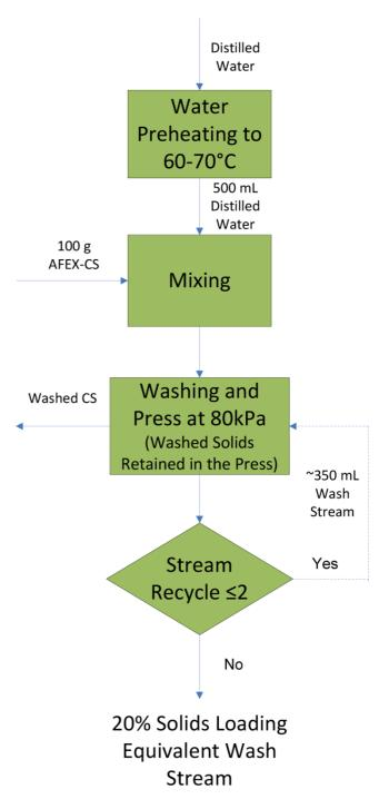
Figure I Schematic describing the preparation of ammonia fiber expansion-corn stover water extract.
