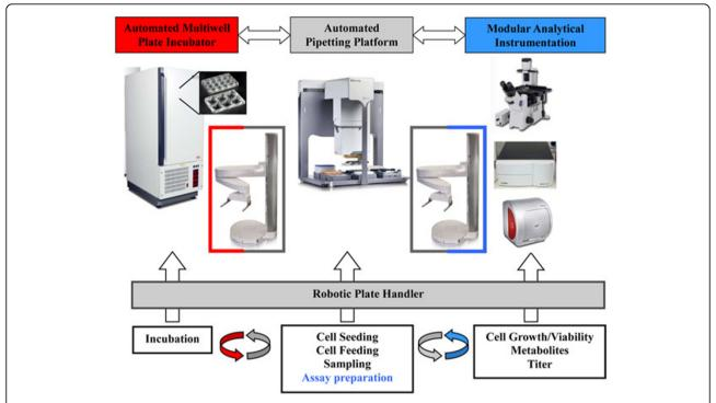
**Figure 1** Schematic illustration of the developed robotic screening system prototype. Only the core system is shown with a robotic plate handler as key device connecting shaken cultivation, processing and analytical components.
