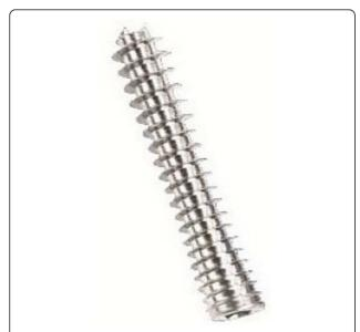
**Figure 2** The Acutrak 2 screw has a head diameter of 4.1 mm and a tip diameter of 4.0 mm. The variable thread pitch causes the screw to advance through the two bone fragments at different rates, causing gradual compression.
