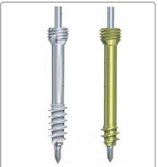
Figure 1 The Synthes 3.0 mm headless compression screw consists of a threadless central shaft with threads of differential pitch at either end promoting fracture compression. Screws are available in long and short threaded
