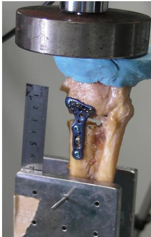
Figure 3 A Material Testing Machine. A Material Testing Machine (Autograph, Shimadzu, Kyoto, Japan) load frame was mounted on the flat of polymethyl methacrylate surface on the metacarpal bones of each specimen with the wrist at full extension. Each specimen was loaded at a constant rate of 20 mm/min to failure under compression.
