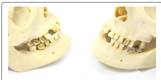
Figure 2 Dental implants are a typical cause of head and neck metal artifacts. A human skull was used as a 'worst case' test object for metal artifact reduction. It features no less than six separate metal foreign bodies: a full gold bridge, a full steel bridge, and four full gold crowns.
