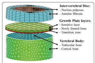
**Figure 1** The detailed modeling of intervertebral disc, growth plate layers, and the vertebral body in the spinal column model.
