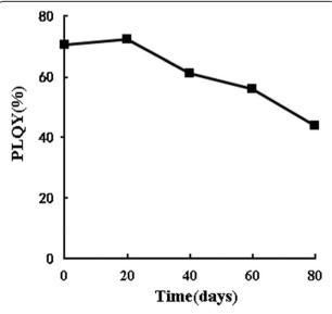
Figure 2 PLQY transformation of CdTe/ZnS aqQDs in situ (pH 8.3) for periods up to 80 days.
