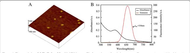
**Figure 1 Characteristics of CdTe/ZnS aqQDs: (A) AFM image, (B) absorption and emission spectra.** The average size was 19.3 ± 2.2 nm in diameter. The maximal emission was observed at approximately 652 nm following excitation at 350 nm.
