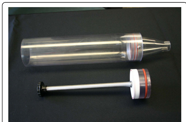
Figure 2 Ferret holder. Shown are the ferret restraint tube with integral connector cone (above) and push rod ["plunger"] (below).
