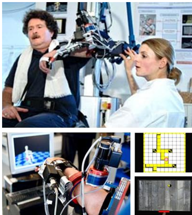
Figure 2 Subject in the robot ARMin II with labyrinth and ball game scenario.
