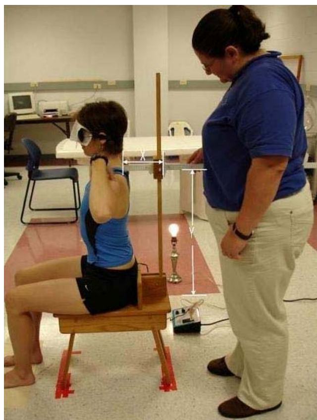
Figure 1 The new measurement method: X and Y coordinates are measured and used in a trigonometric calculation to determine the starting angle. An individual is shown seated in the upright starting posture; during the study, all subjects were blindfolded throughout testing.
