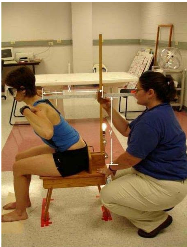
Figure 2 The new measurement method: The X and Y coordinates are shown above with an individual in a position 2/3 of full flexion; during the study, all subjects were blindfolded throughout testing.
