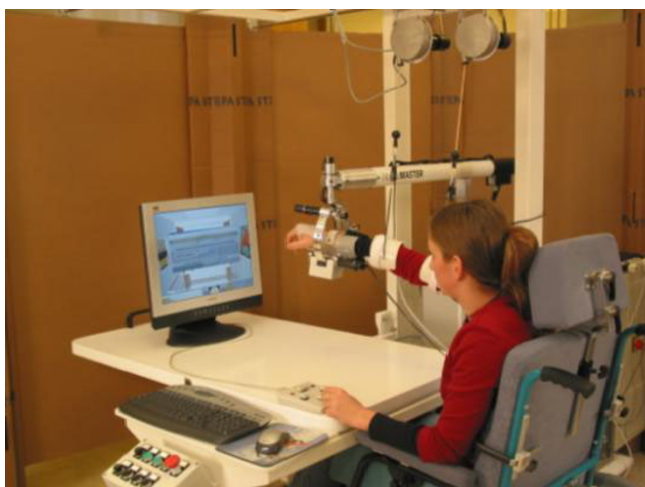
Figure 2 Precursor commercial incarnation of GENTLE/S. This figure depicts the controls for wheelchair docking, and controlling the arm support forces on the left. Patient controls are seen under the subject's left hand and a therapy can be chosen or halted and will only proceed if the 'operate' button is held down. The patient can 'eject' their arm from the HapticMaster.
