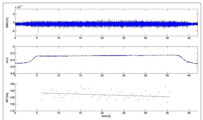
Figure 1 This figure provides an example of the raw signal quality of both the surface electromyogram (upper box) and the accelerogram (mid box) recorded from the L5 left electrode site during an 80% MVC sustained back extension. In the lower box, results of the MF-EMG processing including the MF EMG values calculated for each individual epoch and those of the linear regression analysis are provided.
