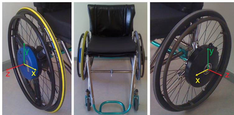
Figure 1 Smartwheel a (left) and Optipush b (right). Both wheels measure three-dimensional forces and torques on the handrim, combined with the angle under which the wheel is rotated. The local coordinate systems are defined as: x- and y-axis, orthogonal to each other in the plane of the handrim, z axis orthogonal to the plane of the handrim and protruding from the wheel axle. The direction of positive torque is mirrored for the wheels so that they measure positive torque when pushing forward.
