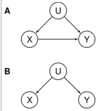
**Figure 1 DAG demonstrating the ideas of confounding**. A: U is an unobserved confounder for the association between X and Y and X is a cause of Y. B: U is an unobserved confounder for the association between X and Y but X is not a cause of Y. From purely observational data these two situations cannot be separated.
