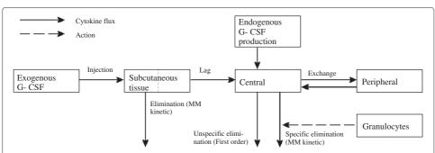
**Figure 2 (Model structure of the pharmacokinetic model of G-CSF).** The major compartments, cytokine fluxes and regulations are presented (MM = Michaelis Menten kinetic). The subcutaneous compartment is divided into two subcompartments with first order transition.
