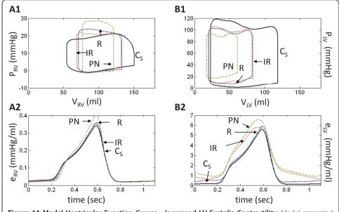
**Figure 11 Model Ventricular Function Curves - Increased LV Systolic Contractility.** Model-generated ventricular function curves of LVDD *with* increased LV systolic contractility. Abbreviations are as in Figure 3.  $C_S$  represents a new elastance control curve where the ESPVR contractility has been augmented, but no other changes have been made.
