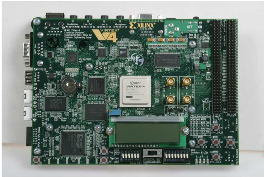
Figure 9 Xilinx ML403 evaluation board used for implementation the proposed algorithm.
