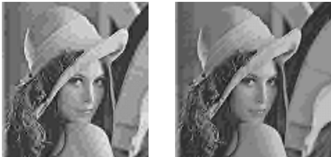
(a): PSNR=26.68 dB, SSIM=0.734, VSNR=15.73 dB (b): PSNR=26.70 dB, SSIM=0.747, VSNR=15.94 dB
