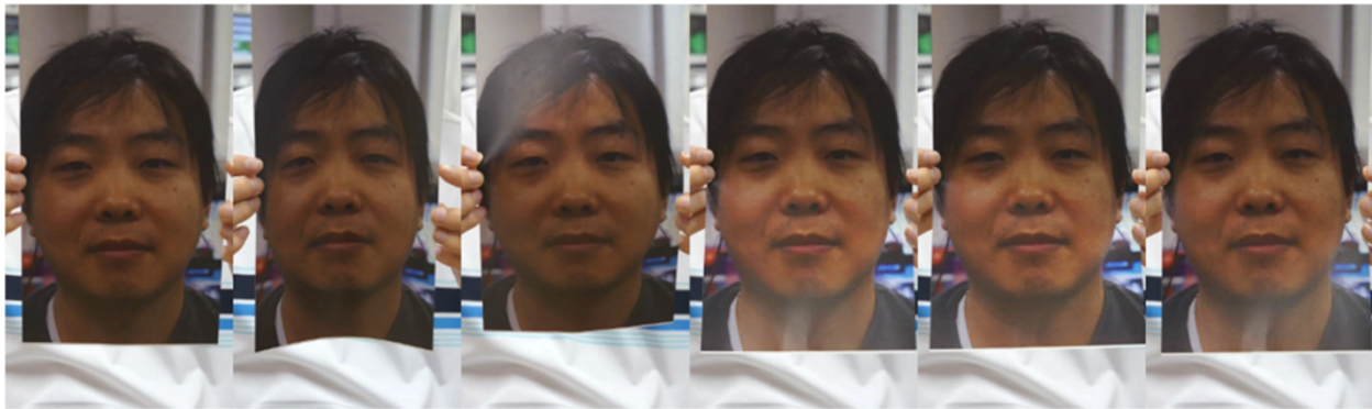
Figure 2 Example sequence of a warped photo attack from the CASIA Face Anti-Spoofing Database [6]. This describes the characteristic reflections (flickering) of a planar spoofing medium and the distorted motion patterns.
