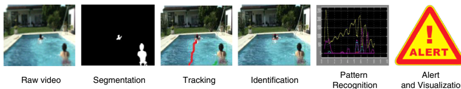
Figure 19 Activities sequence of the early drowning detection at domestic swimming pools.
