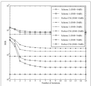
**Figure 3 Convergence of data detection, QPSK,**  $Nf_dT_s = 0.15$ . Convergence performance of the proposed EM-based scheme in Section 3 (marked as scheme 1) and the proposed EM-based scheme in Section 4 (marked as scheme 2) with signal-to-noise ratio (SNR) equal to 10, 20, and 30 dB.
