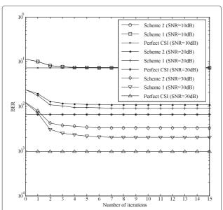
**Figure 2 Convergence of data detection, QPSK,**  $Nf_dT_s = 0.075$ . Convergence performance of the proposed EM-based scheme in Section 3 (marked as scheme 1) and the proposed EM-based scheme in Section 4 (marked as scheme 2) with signal-to-noise ratio (SNR) equal to 10, 20, and 30 dB.
