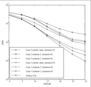
Figure 7 Performance of data detection for different channel length, QPSK,  $Nf_dT_s=0.075$ . BER performance achieved by the proposed iterative algorithm versus SNRs.
