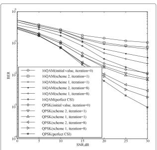
**Figure 5 Performance of data detection, QPSK and 16 QAM,**  $Nf_dT_s = 0.075$ . BER performance achieved by the proposed iterative algorithm versus SNRs.
