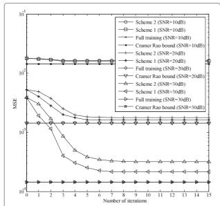
Figure 1 Convergence of channel estimation, QPSK,  $Nf_dT_s = 0.075$ . Convergence performance of the proposed EM-based scheme in Section 3 (marked as scheme 1) and the proposed EM-based scheme in Section 4 (marked as scheme 2) with signal-to-noise ratio (SNR) equal to 10, 20, and 30 dB.
