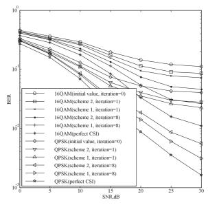
Figure 6 Performance of data detection, QPSK and 16 QAM,  $Nf_dT_s = 0.15$ . BER performance achieved by the proposed iterative algorithm versus SNRs.
