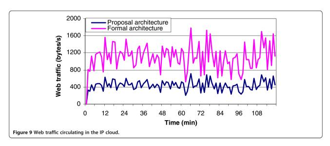
Figure 9 shows the Web traffic circulating in the IP cloud of our simulation. We can observe the behavior of our architecture compared to a normal architecture. Note that the average Web traffic in our proposal is around 430 bytes, compared to the traffic when using a conventional architecture, where the average is around 1090 bytes. Therefore, a 61% improvement is displayed. What is more, we observe that in our architecture the traffic is more stable and displays fewer fluctuations.
