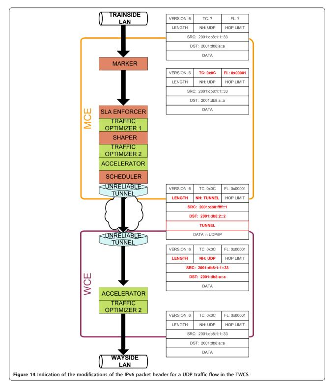
flows. The source IP address of the new packet is the IP address of the wireless interface, which is here assumed 2001:db8:ffff::1 (see Figure 9) and the destination address is the IP address of the WCE, which is here assumed 2001:db8:2::2 (see Figure 9).
