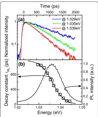
**Figure 4** Temporal evolution of PL intensity and dependence of decay time constant. (a) Temporal evolution of PL intensity at different energies of detection. (b) Dependence of decay time constant versus energy together with time-integrated TRPL spectra.
