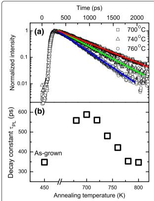
**Figure 1 PL decay curves and decay time constants. (a)** PL decay curves (taken at the maximum of PL emission) for samples annealed at three different temperatures. There is a clearly visible influence of the annealing temperature on the decay rate. Lines represent single exponential fit. **(b)** Decay time constants for all structures.
