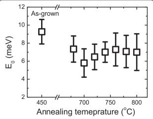
Figure 5 Average energy of localized states  $E_0$  as a function of annealing temperature.
