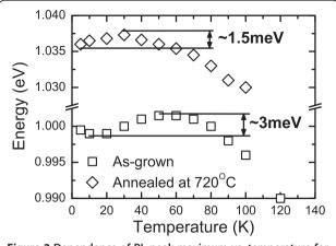
Figure 2 Dependence of PL peak maximum vs. temperature for as-grown (square) and annealed (720°C) (diamond) GalnNAsSb QW samples.
