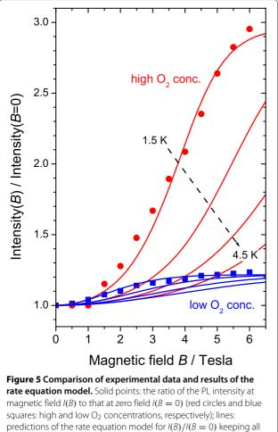
predictions of the rate equation model for l(B)/l(B = 0) keeping al parameters constant except those related to the oxygen concentration and for a series of temperatures (upper to lower curves) of 1.5 to 4.5 K in 1-K steps.
