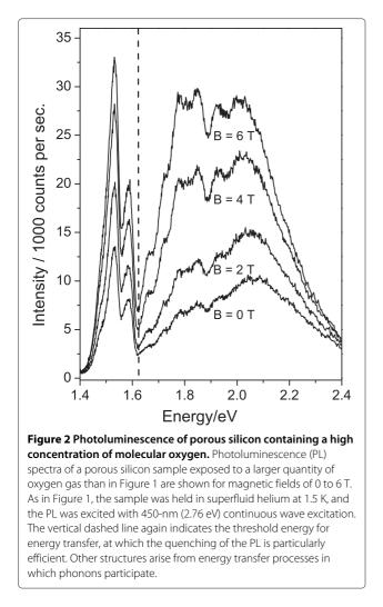
Figure 2 demonstrates that significant PL is again observed above the threshold for energy transfer to oxygen, even at this higher oxygen concentration. Furthermore, the PL both above and below this threshold shows a much stronger recovery of intensity as the magnetic field is increased, by factor of about 3 times, and unlike the case of Figure 1, the recovery of the PL has not saturated up to a magnetic field of 6 T.
