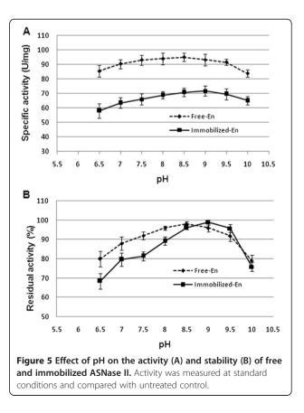
after 24-h incubation at  $4^{\circ}C \pm 1^{\circ}C$  showed that the free ASNase II retained the maximum of its original activity between pH 8.0 and 9.0 and about 80% at pH 10. The immobilized ASNase II retained about 100% activity at pH 9.0 and about 75% at pH 10.
