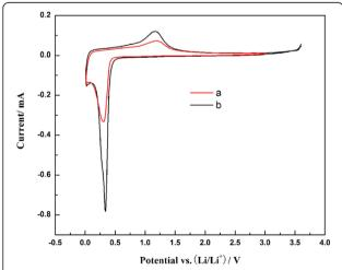
**Figure 5 Cyclic voltammograms of MnO<sub>2</sub> materials.** After five charging-discharging cycles measured at a scan rate of 0.05 mV s  $^{-1}$ in the potential range of 0.01  $\sim$  3.60 V. **(a)** Caddice-clew-like and **(b)** urchin-like MnO<sub>2</sub> samples.
