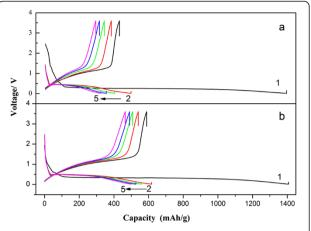
Figure 4 Charge-discharge specific capacity-voltage curves of  $MnO_2$  anode materials in the potential range of 0.01 ~ 3.60 V at 0.2 C. (a) Caddice-clew-like and (b) urchin-like  $MnO_2$  samples.
