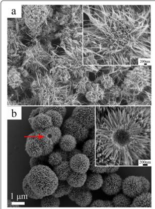
Figure 1 SEM images of  $MnO_2$  samples obtained under (a) neutral and (b) acidic conditions. The scale bar is 1  $\mu$ m. The inset shows the enlarged SEM image of  $MnO_2$  sample and the scale bar is 200 nm.
