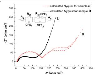
**Figure 6 Nyquist plot of Li/MnO<sub>2</sub> cells after five charging and discharging cycles at open circuit voltage.** The frequency ranged from 0.1 Hz to 100 kHz with an applied AC signal amplitude of 5 mV. **(a)** Caddice-clew-like and **(b)** urchin-like MnO<sub>2</sub> samples. Symbols represent experimental data and lines represent fitted spectra using equivalent circuit. The inset is the equivalent circuit.
