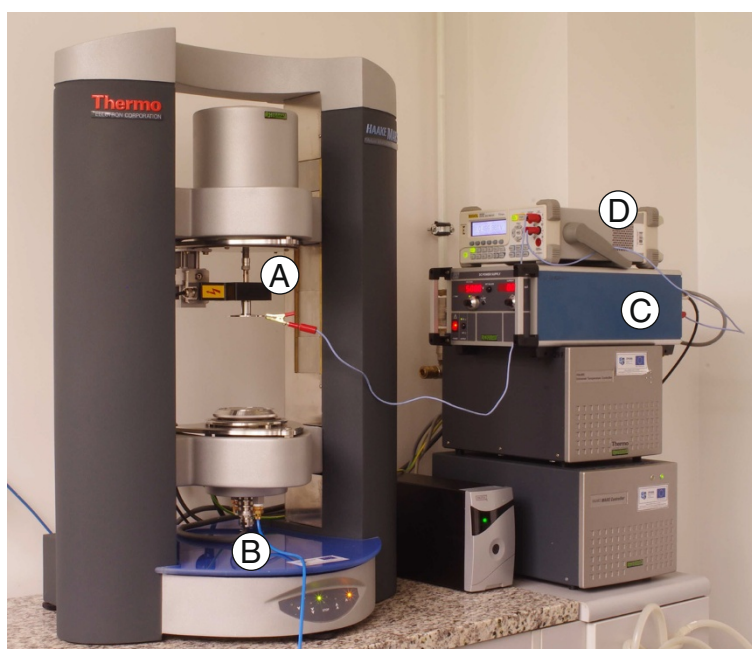
Figure 4 System used to study rheological properties in electric field at position before measurement – validation of system. (A) a transfer element connection to the rotor through a ball bearing, (B) compressed air supply line to the cooling system rheometer, (C) a voltage generator, (D) multimeter.
