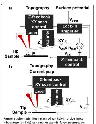
measurements. A lock-in amplifier was operated with a sensitivity of the 100 mV/nA.
