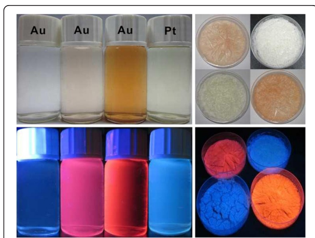
Figure 1 Photographs of luminescent metal clusters in the form of solution and solid states. Under natural light and UV irradiation ( \lambda = 365 nm).
