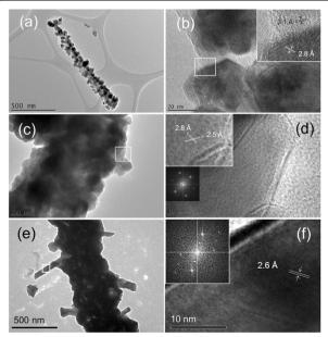
**Figure 4 HRTEM** analysis on the Si/ZnO heterostructure NWs. TEM and HRTEM micrographs of Si/ZnO core-shell NWs prepared at different ZnO growth time of (**a**, **b**) 0.5, (**c**, **d**) 1, and (**e**, **f**) 1.5 h. Magnified HRTEM micrographs from (**b**) and (**d**) are inserted in the respective figures. FFT patterns inserted in (**d**) and (**f**) are converted from the appropriate HRTEM micrographs.
