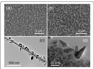
**Figure 1 SEM and TEM studies on the In/Si NWs.** FESEM images of **(a)** Si NWs and **(b)** In seeds coated on Si NWs. **(c)** TEM and **(d)** HRTEM micrographs of the In seeds coated on the surface of the Si NW
