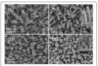
Figure 2 Morphology study of the ZnO nanostructures grown on In/Si NWs. FESEM images of ZnO nanostructures formed on In/Si NWs at different growth times of (a) 0.5, (b), (c) 1.5, and (d) 2 h. Insets in (b) and (d) are the cross-sectional images of the respective figures (scale bar = 1  $\mu$ m).
