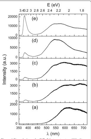
**Figure 6 PL analysis on the Si/ZnO heterostructure NWs.** PL spectra of **(a)** In/Si NWs and Si/ZnO core-shell NWs prepared at different ZnO growth times of **(b)** 0.5, **(c)** 1, **(d)** 1.5, and **(e)** 2 h.
