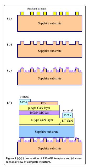
materials. Wet etching is divided into mask-associated etching and mask-free etching [10-12]. Mask-associated etching utilizes a circular array of  $\mathrm{SiO}_2$  on the surface of a sapphire substrate as an etching barrier layer. The mask-free etching process uses the by-product of the reaction between the chemical etching solution and the etched material as the etching mask. However, the use of a patterning process without an additional photolithographic step can reduce manufacturing cost.
