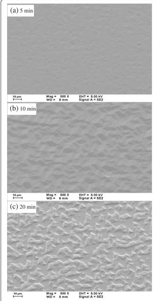
Figure 3 FESEM images of sapphire substrate following etching in phosphoric acid for various times.
