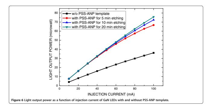
dispersed on the patterned surface of the PSS, forming the PSS-ANP template. The mean particle size was approximately 400 nm. The PSS-ANP template in the GaN-based LED structure scattered and reflected the back-emitted light from the active layer of the LED.
