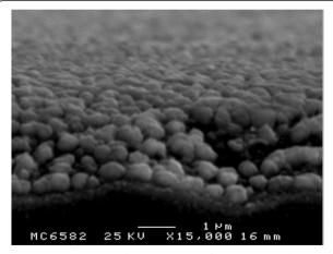
Figure 4 Cross-sectional FESEM image of PSS-ANP template with annealing at 500°C and etched for 5 min.
