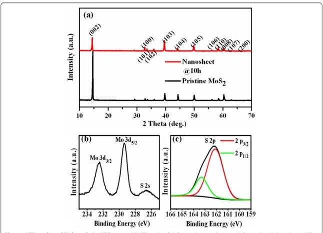
**Figure 1 XRD results and high-resolution XPS spectra. (a)** XRD results of  $MoS_2$  nanosheets and pristine  $MoS_2$  powders. High-resolution XPS spectra of **(b)** Mo 3*d* and **(c)** S 2*p* for the exfoliated  $MoS_2$  nanosheets (10 h).
