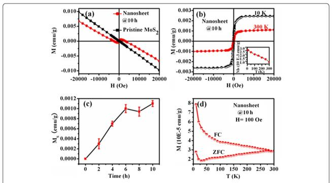
**Figure 4 Room-temperature** *M-H*, **ZFC**, **and FC curves**. **(a)** Room-temperature *M-H* curves for MoS<sub>2</sub> pristine powders and nanosheets. **(b)** *M-H* curves for MoS<sub>2</sub> nanosheets measured at 10 and 300 K: the DM signals of the samples have been deducted. **(c)** The dependence of the saturation magnetization of the MoS<sub>2</sub> nanosheets on sonication time. **(d)** The ZFC and FC curves for the exfoliated MoS<sub>2</sub> nanosheets sonicated in DMF for 10 h.
