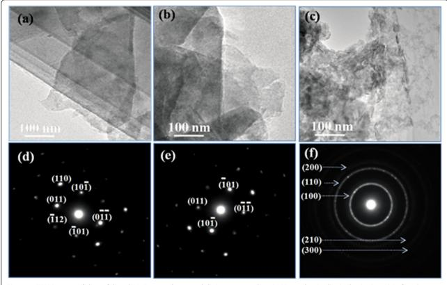
Figure 2 TEM images of the exfoliated MoS<sub>2</sub> nanosheets and their corresponding SAED results. (a, d) 2 h, (b, e) 4 h, and (c, f) 10 h.
