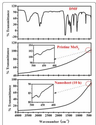
**Figure 6 FTIR patterns.** FTIR patterns of the solution DMF, the pristine  $MoS_2$  powder, and the  $MoS_2$  nanosheets sonicated in DMF for 10 h.
