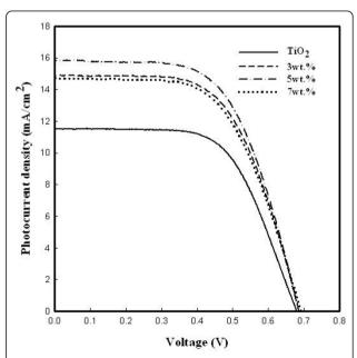
Figure 6 Photocurrent-voltage curve of the  $TiO_2$  film and the  $TiO_2$  films with  $ZrO_2$  nanofibers.
