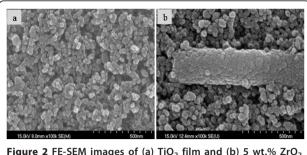
Figure 2 FE-SEM images of (a)  ${\rm TiO_2}$  film and (b) 5 wt.%  ${\rm ZrO_2}$  nanofiber-doped  ${\rm TiO_2}$  film.
