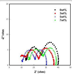
**Figure 5 Nyquist plots of the DSSCs using TiO<sub>2</sub> film and ZrO<sub>2</sub> nanofiber-doped TiO<sub>2</sub> film.** Black circle, 0 wt.%; red diamond, 3 wt.%; cross mark, 5 wt.%; green triangle, 7 wt.%.
