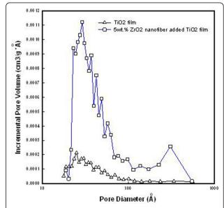
Figure 3 BJH curve of TiO<sub>2</sub> film (triangle) and 5 wt.% ZrO<sub>2</sub> nanofiber-doped TiO2 film (square).
