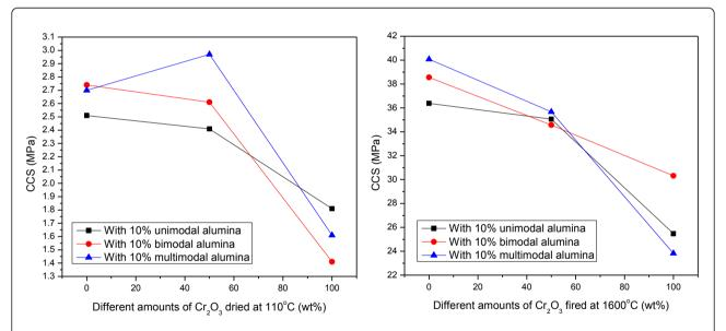
Figure 3 Effects of adding ultrafine active alumina on the cold crushing strength of the castables. The castables were subjected with different amounts of  $Cr_2O_3$  at temperatures of 110°C and 1,600°C.
