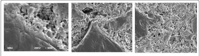
Figure 4 The variation of microstructures of castables due to the different ultrafine alumina powders in matrix. (a) Unimodal alumina, (b) bimodal alumina, and (c) multimodal alumina.
