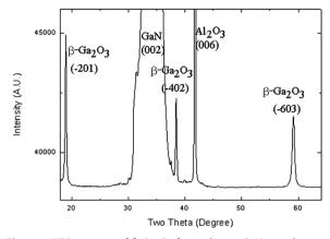
Figure 1 XRD pattern of  $\beta\text{-}Ga_2O_3$  formed on a GaN template for sample III
