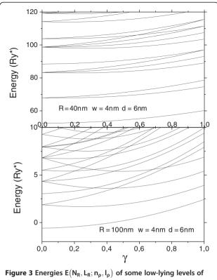
Figure 3 Energies  $E(N_R,L_R;n_\rho,l_\rho)$  of some low-lying levels of the double-donor complex in vertically coupled QDs. As functions of the magnetic field.
