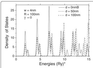
**Figure 5** Density of states for three different distances between layers. Corresponding to low-lying levels of the double-donor complex in vertically coupled QDs.
