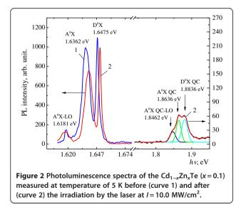
the blue shift of  $A^0X$  and  $D^0X$  exciton bands - due to photo-induced mechanical compressive stress of the top layer.
