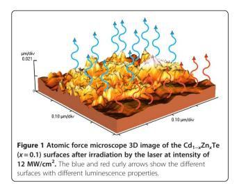
strongly absorbed Nd:YAG laser radiation with intensity of  $I = 12.0 \text{ MW/cm}^2$  was observed using AFM, as shown in Figure 1.
