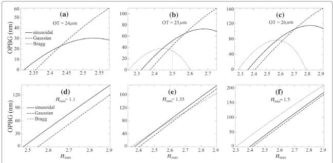
**Figure 1 OPBG as a function of**  $n_{max}$  **for the sinusoidal, Gaussian, and Bragg profiles.** Panels (**a**), (**b**), and (**c**) correspond to the OT of 24, 25, and 26  $\mu$ m, respectively. Panels (**d**), (**e**), and (**f**) correspond to the PT = 7.76  $\mu$ m for three different values of minimum refractive index. The OPBG was computed between 0° and 85° of incidence angle at 99% of the reflectivity.
