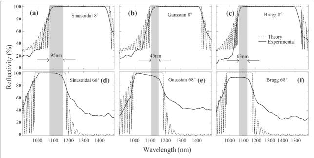
**Figure 2** Theoretical (dashed line) and experimental (solid line) reflectivity spectra for structures with the same OT. The PBG generated using the (a) sinusoidal, (b) Gaussian, and (c) Bragg profiles for 8°. The corresponding reflectivity spectra at 68° are shown in panels (d), (e), and (f), respectively. The overlapping of the experimental PBG between 8° and 68° is shown as a gray band (taken for the reflectance more than or equal to 90%).
