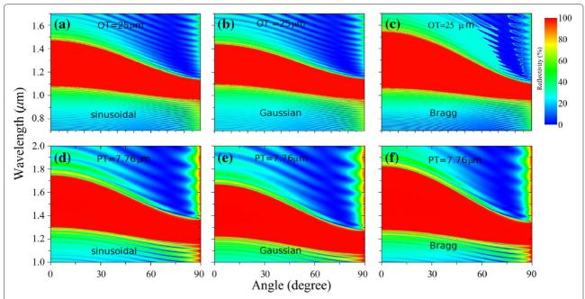
Figure 4 Contour plot of the reflectivity spectra as a function of the angle and wavelength. (a, d) Sinusoidal, (b, e) Gaussian, and (c, f) Bragg refractive index profiles. The color scale indicates the reflectivity percentage from 0% (blue) to 100% (red).
