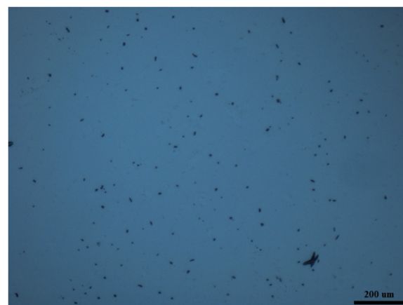
Figure 4 Optical image of graphene/[HMIM]BF 4 Ionanofluid (0.03 wt.%).
