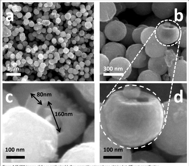
Figure 3 FE-SEM images of the as-synthesized hollow magnetite microspheres obtained at different magnification.
