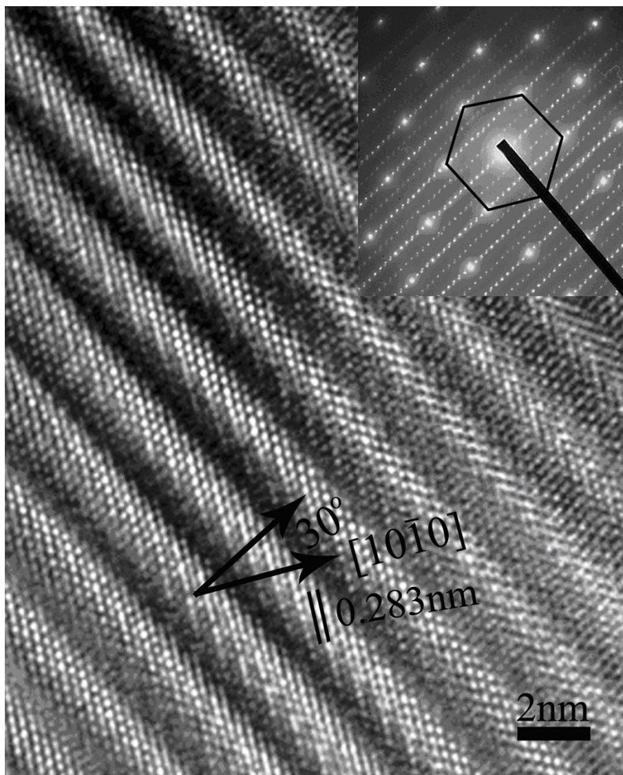
Figure 3 HRTEM image of the superlattice structure. The inset of the figure shows the corresponding SAED pattern in the brightfield part of the leaf-like nanostructure.
