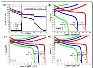
**Figure 2** Discharge capacities, cyclic performances, and discharge profiles of the thin films. (a) Discharge capacities and cyclic performances of pristine and fluoride-coated LiCoO<sub>2</sub> thin films, (b) discharge profile of the pristine film, (c) discharge profile of the AlF<sub>3</sub>-coated film, and (d) discharge profile of the LaF<sub>3</sub>-coated film. (The voltage was in the range of 4.25 to 3.0 V, and the current densities were 0.2, 0.4, and 0.6 mA· cm<sup>-2</sup>.).
