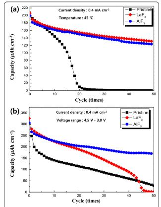
**Figure 3 Cyclic performances of the pristine and fluoride-coated LiCoO₂ film electrodes.** (a) Cyclic performances measured at 45°C in the voltage range of 4.25 to 3.0 V at a current density of approximately 0.4 mA· cm<sup>-2</sup> and (b) measured at 30°C in the voltage range of 4.5 to 3.0 V at a current density of approximately 0.4 mA· cm<sup>-2</sup>.
