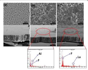
**Figure 1 SEM images of the pristine and coated LiCoO<sub>2</sub> thin film electrodes.** (a) Pristine film, (b) AlF<sub>3</sub>-coated film, and (c) LaF<sub>3</sub>-coated film. The bottom of the figure shows EDS peaks of the surface of the coated samples.
