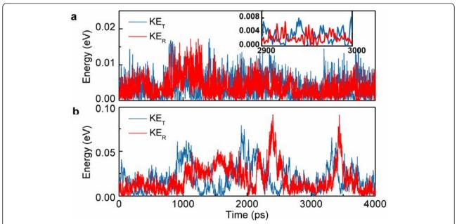
Figure 3 Conversion between the translational and rotational kinetic energies of  $C_{60}$  during surface diffusion on the graphene. The temperatures are (a) T = 50 K, and (b) T = 200 K. The inset of (a) shows the interplay between the translational and rotational energies as a function of time at T = 50 K with a higher resolution.
