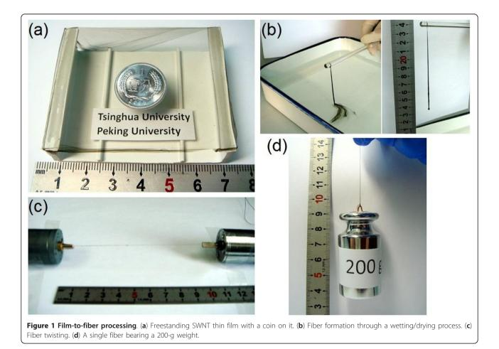
process allowed one-step formation of continuous nanotube fibers.
