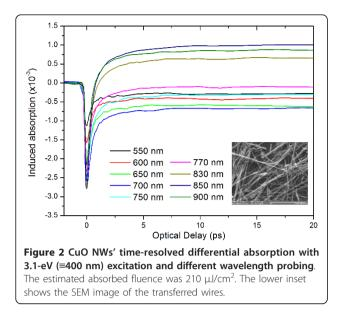
limited) in optical absorption reaching a minimum, followed by a fast recovery toward a plateau within 5 to 10 ps, and then returning back to its equilibrium value over several nanoseconds.
