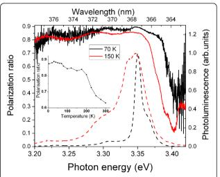
Figure 4 Polarization ratio of the PL emission from one of the analyzed nanowires. As a function of the photon energy for temperatures  $T=70~\rm K$  (full black curve) and 150 K (full red curve). The normalized PL spectra recorded at  $T=70~\rm K$  (dashed black curve) and 100 K (dashed red curve) are reported as reference. The inset reports the polarization ratio of the whole spectrum as a function of temperature.
