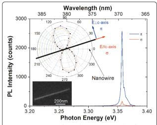
**Figure 3 μ-PL spectra of a single nanowire on carbon-formvar membrane.** Collected at 4.2 K for E // c and  $E \perp c$  with a spectral resolution of 1.5 meV. The polarization diagram and SEM image of a studied nanowire lying on the substrate are reported in the inset.
