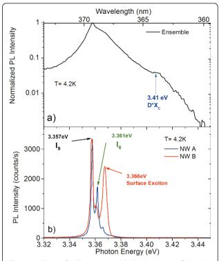
**Figure 2 PL and \muPL spectra**. (a) PL spectrum of the NW ensemble collected at 4.2 K. (b)  $\mu$ PL spectra of two single nanowires (blue and red) collected at 4.2 K with a spectral resolution of 800  $\mu$ eV.
