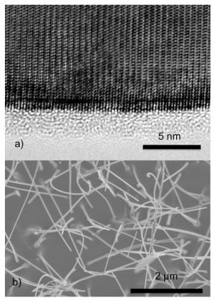
**Figure 1 Bright-field HRTEM and SEM images.** (a) Bright-field HRTEM image along the <11-20 > viewing direction of a ZnO nanowire. (b) SEM image of ensemble of ZnO nanowires.
