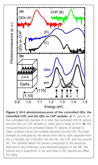
suggests that a significant fraction of excitons are able to combine radiatively. The 1.377-eV peak energy is higher than the bulk  $In_{0.13}Ga_{0.87}As$  bandgap of 1.323 eV and agrees well with the electron and hole eigenenergies estimated from self-consistent solutions of coupled Poisson-Schrodinger equation [29].
