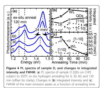
making available more free carriers. Low-temperature hydrogen annealing is a standard Si process that effectively neutralizes interface-trapped charges [37] since hydrogen can diffuse several microns into Si even at room temperature [38].
