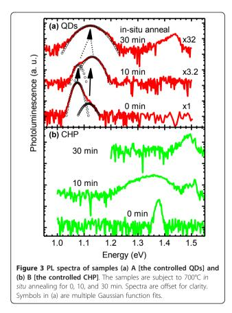
Gaussian function. The bimodal size distribution is thus maintained during the initial stages of annealing but is transformed into a monomodal one after extended annealing.
