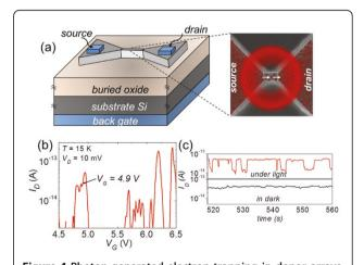
**Figure 4 Photon-generated electron trapping in donor arrays** (a) Device structure of a back-gated SOI-FET for light illumination measurements. With  $V_G$  set on the first observable current peak (b), effects of photon absorption in the nanoscale channel can be observed as RTS in the time-domain measurements (c).
