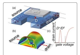
**Figure 1 Operation of a single dopant transistor**. (a) Schematic illustration of a single-donor transistor, in this case a transistor that contains one donor in its nanoscale channel. (b) The conduction path donor mediates single-electron tunneling from source to drain, giving rise to a current peak in the low-temperature transfer characteristics (c).
