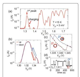
**Figure 3 Single-electron transfer between two donors.** (a) Low-temperature  $I_D$ - $V_G$  characteristics showing a single-donor current peak used as a sensor for detecting charging and discharging of a neighboring donor. (b)-(c) Charging and discharging are sensed as abrupt jumps of the current (producing a hysteresis between upramping and down-ramping curves) and (d) as RTS in the time-domain measurements.
