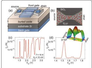
**Figure 2 Single dopants in dopant-rich environment.** (a) Device structure of a phosphorus-doped SOI-FET with the channel containing several donors. (b) SEM image of the channel area with an illustration of random donor arrangement. (c) An example of device characteristics with a single isolated first peak, indicating single-electron tunneling via a donor QD even in a donor-rich channel. (d) Zoom in on the first peak (inset: single-electron tunneling via a donor in a donor-rich channel).
