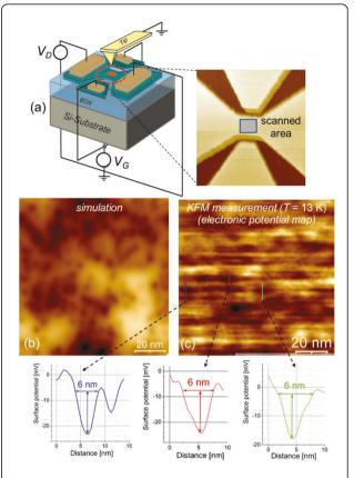
**Figure 5 KFM observation of discrete dopants in device channel.** (a) Setup for LT-KFM measurements, showing in the inset the topography of the measured channel area. (b) Simulated surface electronic potential map due to ionized P donors in a thin Si layer. (c) Measured electronic potential maps at the surface of P-doped SOI-FETs (lower panels are line profiles through some of the dark spots, i.e., regions of lower electronic potential).
