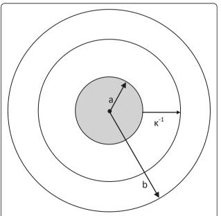
**Figure 1** Schematic of Kuwabara's cell model with particle radius, a, electrical double layer thickness,  $\kappa^{-1}$ , and surrounding shell of liquid medium with outer radius b.
