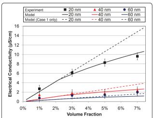
Figure 2 Measured (solid symbols) and predicted (solid lines) electrical conductivity of propylene glycol-based ZnO nanofluids with 20-, 40-, and 60-nm diameter particles.
